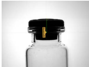
Figure 217. Measure Tool from Edge01 to Measure01
