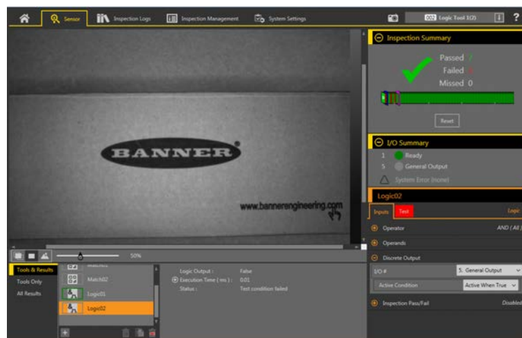
Figure 316. I/O Summary—Large Box Passes with no Output
