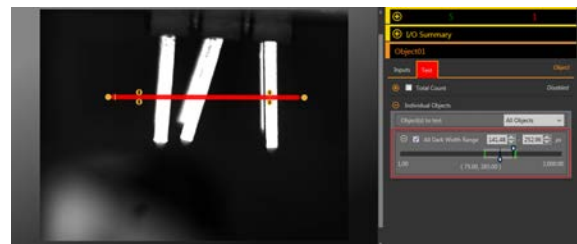
Figure 263. Bad Part—Bent Pin
