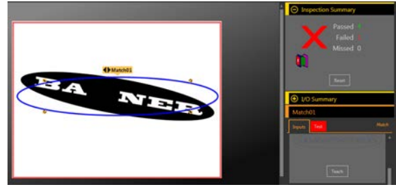
Figure 243. Bad Part—Missing Letter
