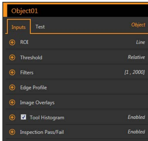
Figure 244. Object Tool—Input Parameters
