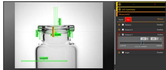
Figure 220. Bad Part—Missing Stopper
