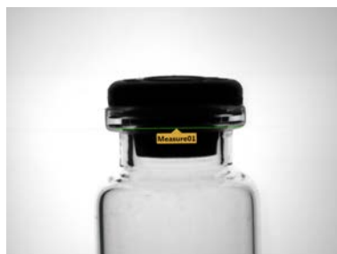
Figure 216. Measure Tool from Edge02 to Edge03
